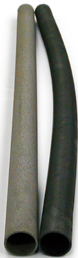
Tubes in Kanthal® APMT (left) and Fe-35Ni-25Cr (right) after the sagging test.
