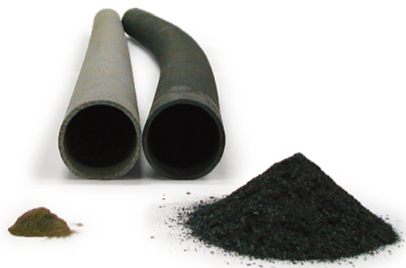
Comparison of Kanthal® APMT tube versus Fe-35Ni-25Cr (after 2300 h at 1100°C [2010°F]). The FeNiCr tube is severely contaminated with oxide flakes.
